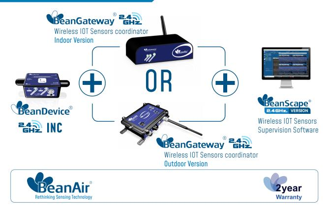
The BeanDevice® 2.4GHz INC operates only on our Wireless IIOT Sensors, you will need the BeanGateway® 2.4GHz and the BeanScape® 2.4GHz for starting a wireless IIOT sensors.
